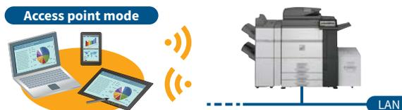
Note: External networks cannot be accessed via the MFD. Up to five mobile devices can be wirelessly connected to the MFD at the same time.
